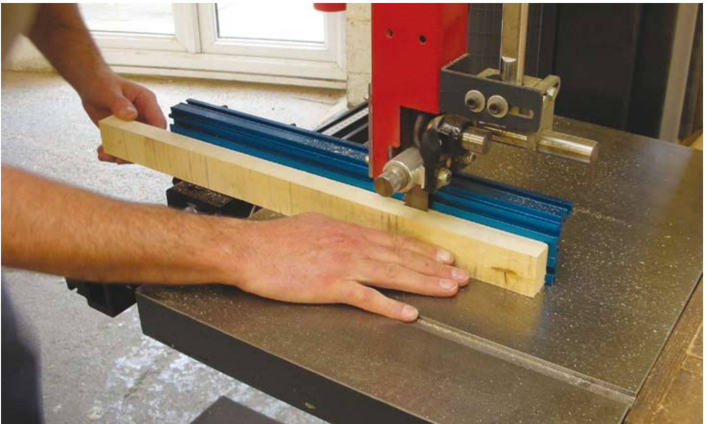
Solid lamina cut on the bandsaw
