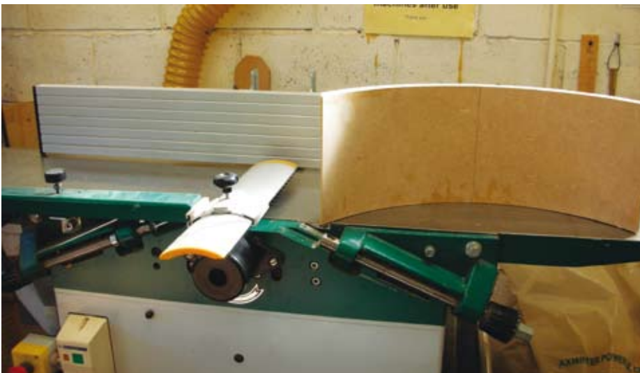
Passing a panel over the planer to achieve a straight edge
