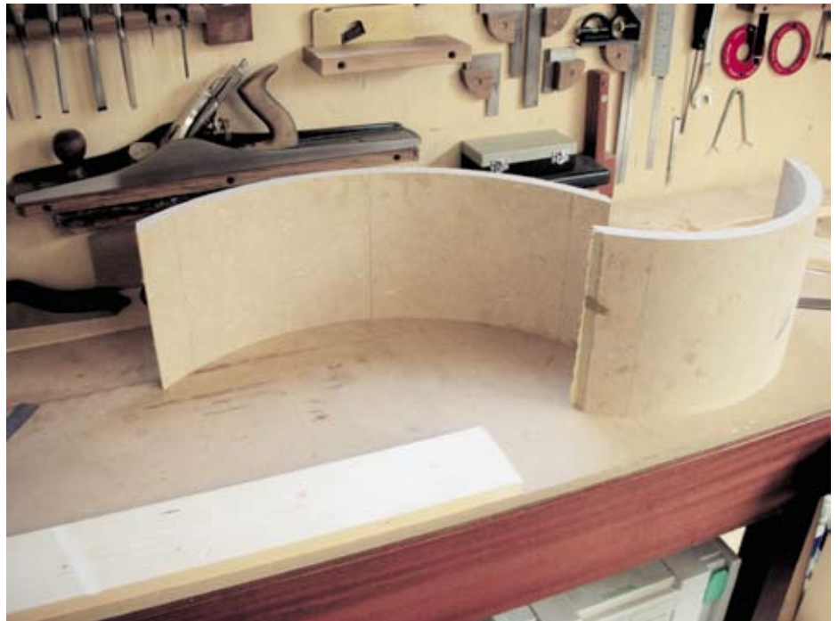
Curved panel made from 2mm MDF lamina
