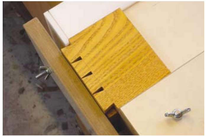
12 Move the tail board forward by enough to offset the scalpel line by its own thickness so the pins are marked on the outside rather than the inside
