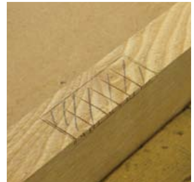
Carefully positioned saw cuts break up the area to be removed
