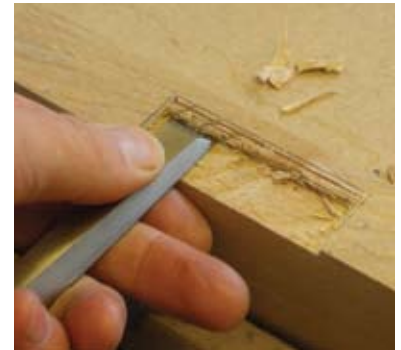
Creep up to your marking lines with a chisel
