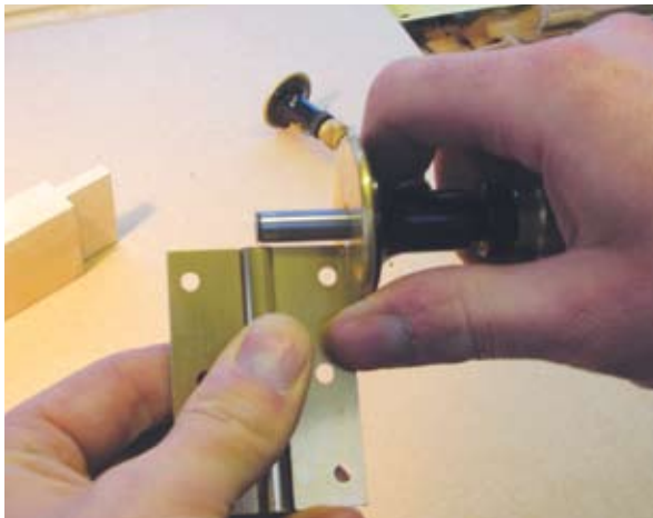
Use a marking gauge to establish the depth of the hinge
