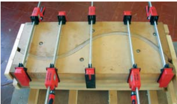
Male and female former laminating is squeezing the lamination between a male and female former made of stacked MDF
