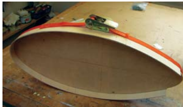
A ratchet strap can be used to tighten up the laminates
