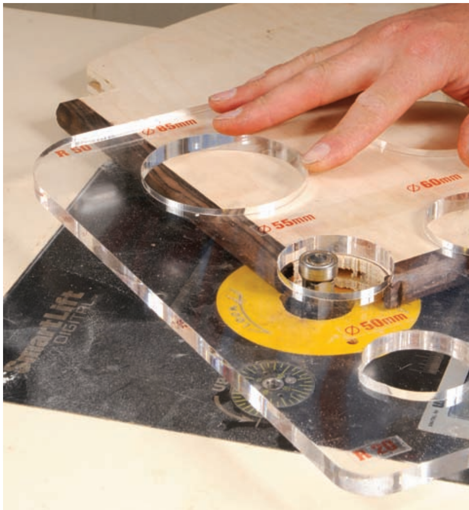
1.3 Use of an acrylic circle-cutting template ensures most of the waste is removed
