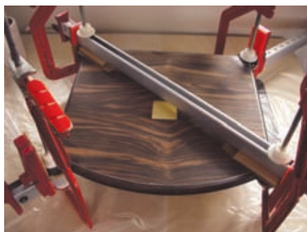
1.8 The setup for clamping the ferrules in place
