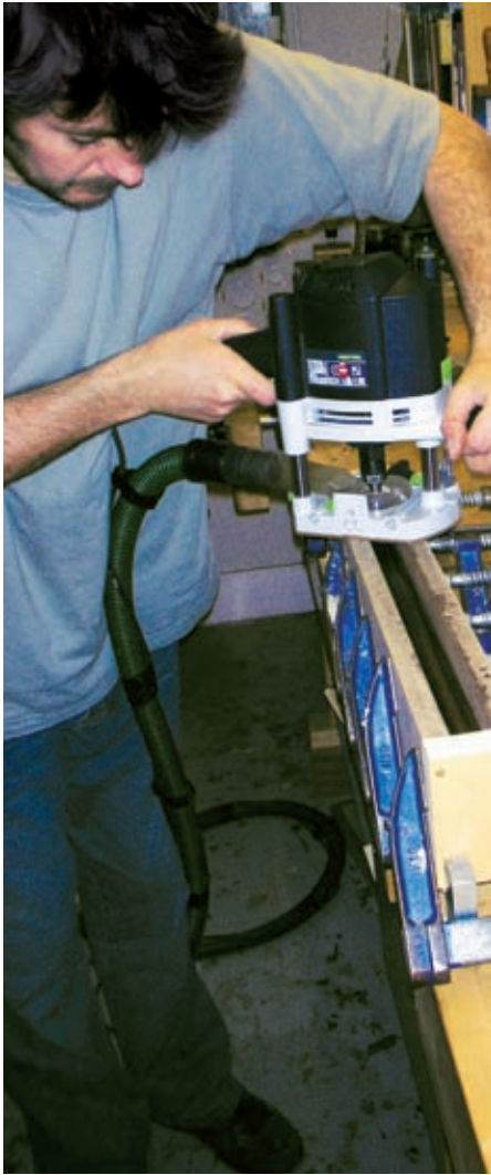
2.1 Using a fluting box to hold the upright while the slot for glass is routed
