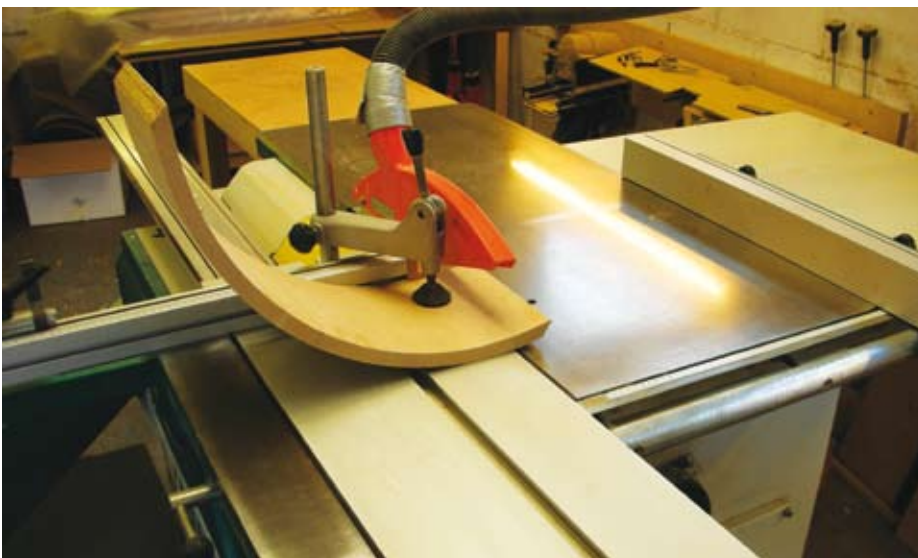
Trimming to size on the dimension saw
