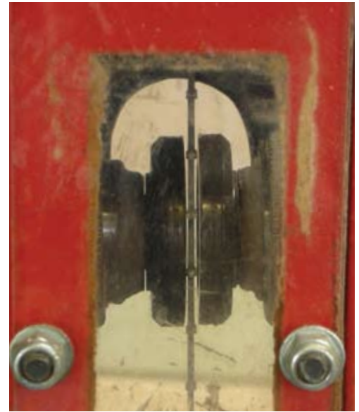
The guides need to be as close as possible but not touching
