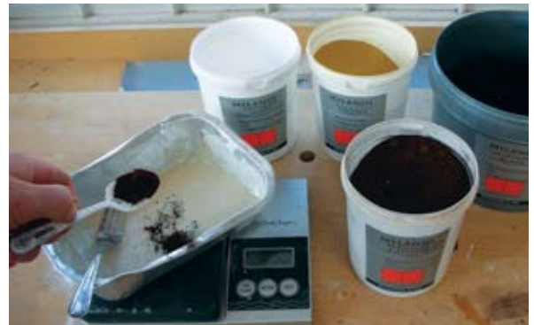
You can tint both urea-formaldehyde and epoxy glues by mixing small quantities of pigment powders
