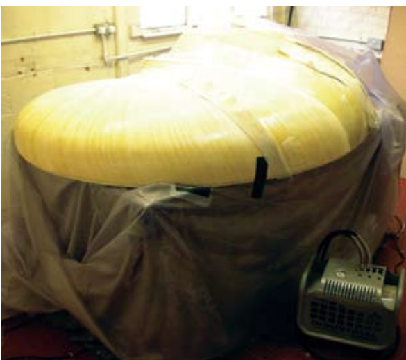
Here I am using our homemade vacuum bag in the production of my 'Nautilus' table
