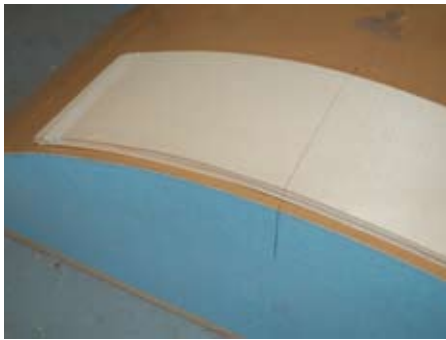
11 The curved back of the drawer has the same radius as the cabinet front
