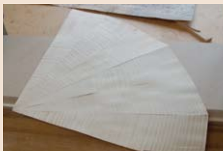
4 ... is joined with UF glue and clamped with Sellotape
