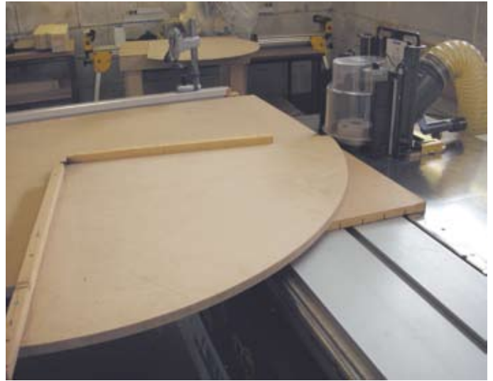
7 The curves for the smaller cabinet were laminated from 2mm material
