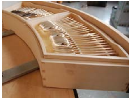
12 The moisture content of the PVA led to the curved pieces cupping so I used UF instead
