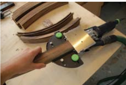
8 The horizontal bands and door rails were veneered over flexi-ply, then laminated again in the vacuum bag
