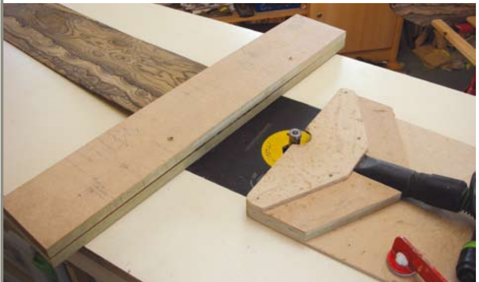
Veneer can be clamped between two layers of MDF and the router bearing run against one of them...
