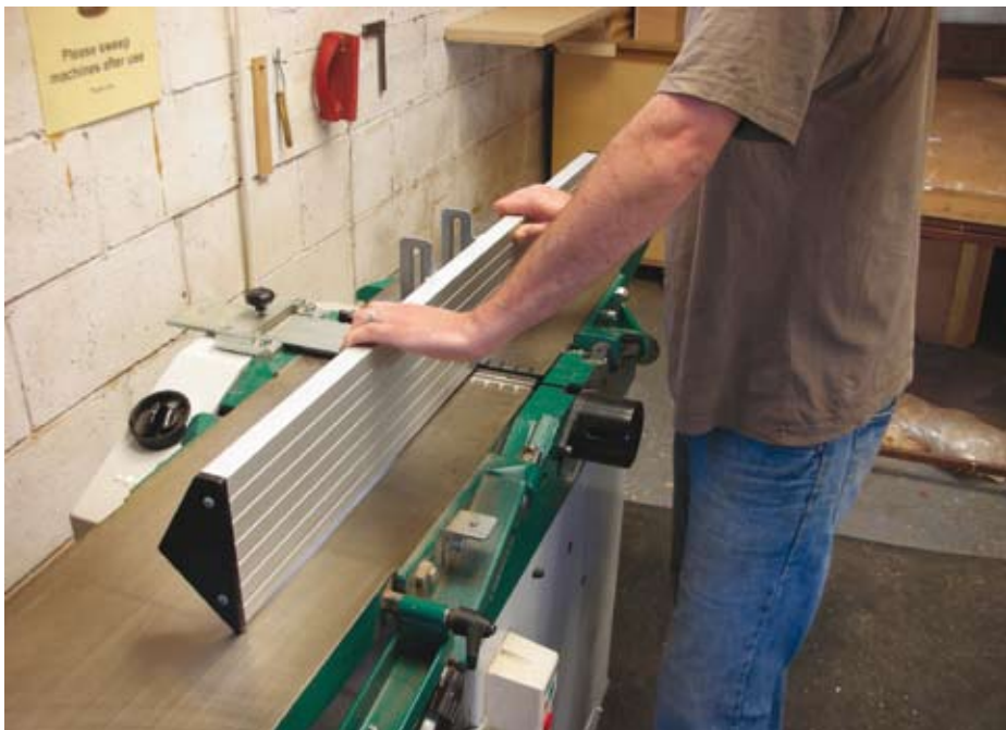
Set up the surface planer like this for tackling short lengths of veneer
