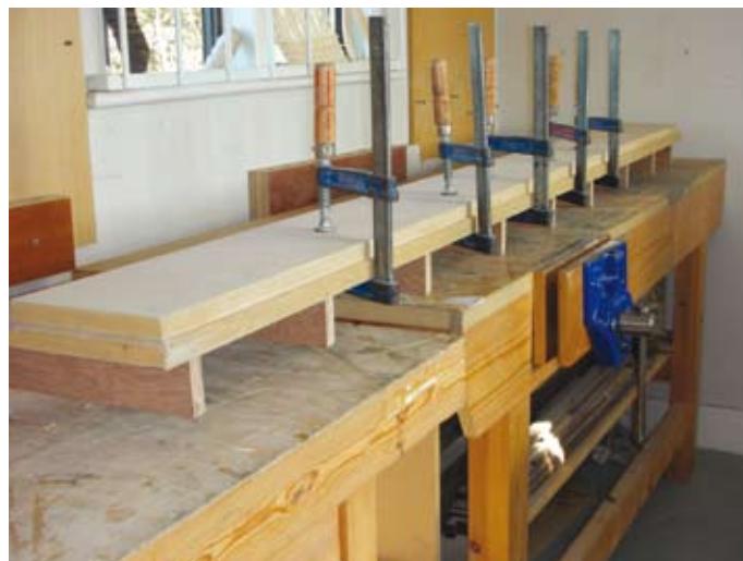
Shooting board clamping assembly
