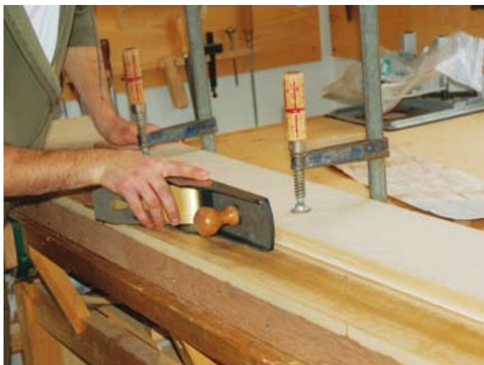
Shooting veneer by hand is not as straightforward as it looks here
