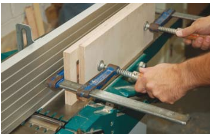
Keep your hands on the clamp handles where they will be nowhere near the rotating cutter...
