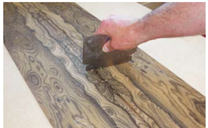
Use a scraper to clean off the excess glue
