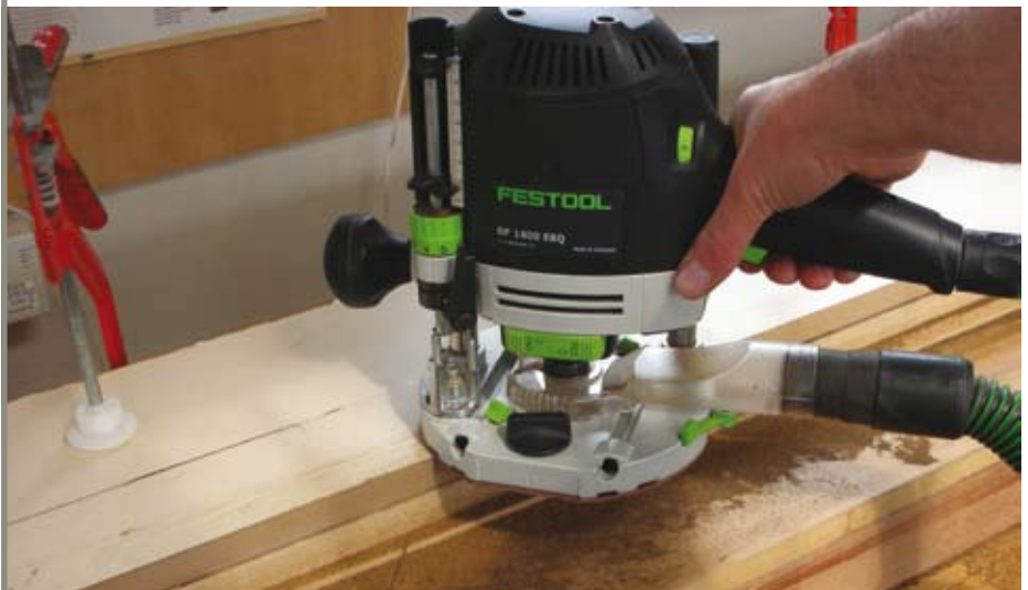
Using a hand-held router to shoot a board
