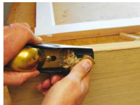
A blockplane does a good job but the going is slow
