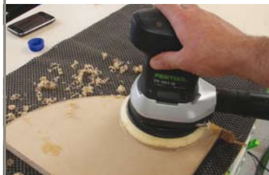
Trimming lipping with a disc sander
