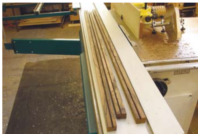
Grooves in lippings cut with a spindle moulder
