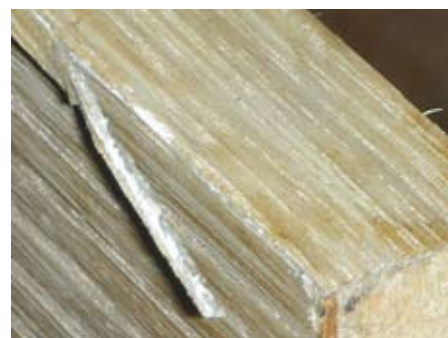
Breakout is always a possibility when using an edger
