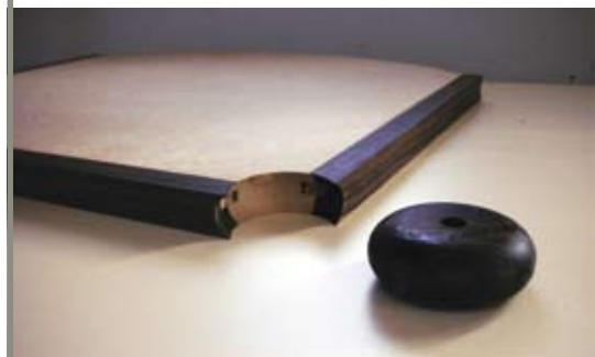
Lipping is applied to the substrate via a loose tongue
