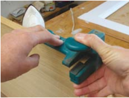
Using an end trimmer on iron-on edging
