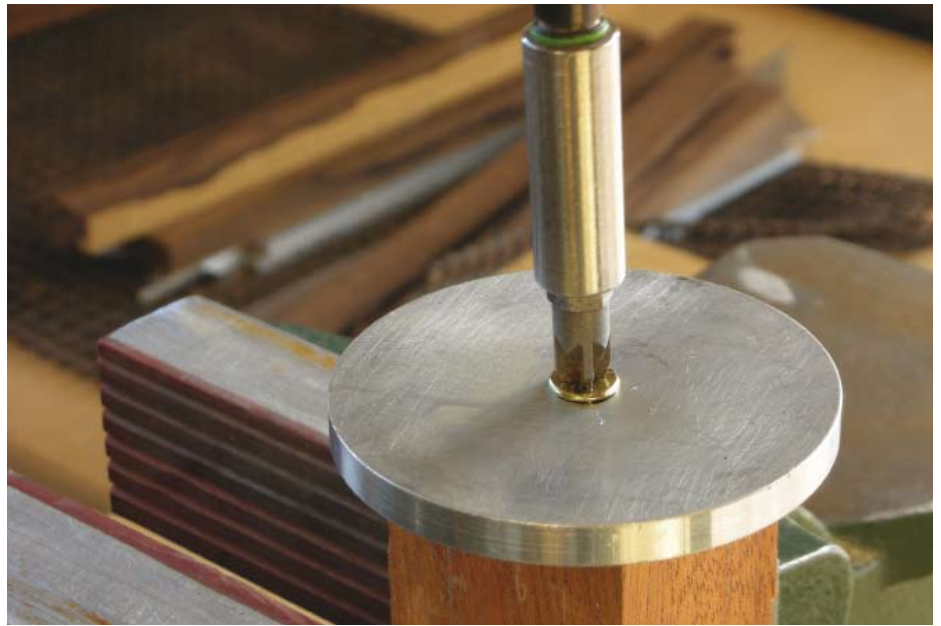
Discs attached to both ends of the stock as guides
