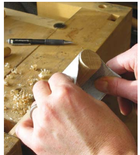
Final stage: sanding to remove the last of the points
