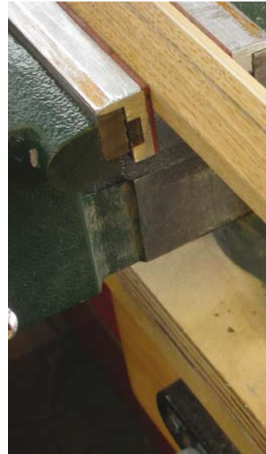
Square section marked out to create an octagon
