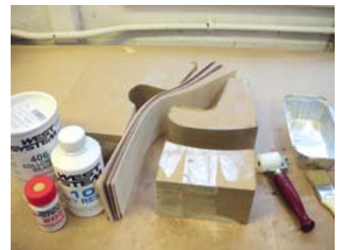
As with any glue-up, preparation is the key to success. Establishing now that our former would have to be in three components to work, will have great influence on how we construct the life size one
