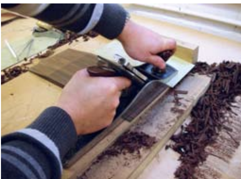
Even a model can benefit from making test pieces. MDF was used to establish the sweeping chamfers and then used to shape the final piece of macassar
