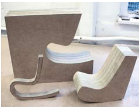
Crude but effective. An MDF template was the starting point for producing the formers. A small band saw with a narrow blade is perfect for working little shapes from what are really no more than off-cuts
