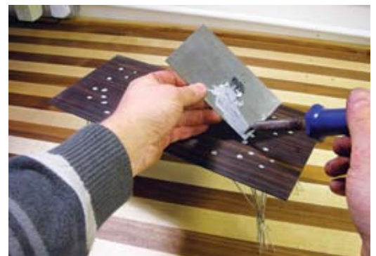
Koniq wax dries hard as it cools so works as an adhesive for model making. It can be mixed to reproduce almost any colour helping to emphasise design details
