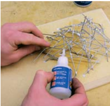
This delicate design is glued to the base to make construction easier
