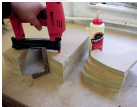
Components for the formers are produced using a router just as they would be for the finished article. At this scale a pin gun provides a quick and cheap solution to assembly
