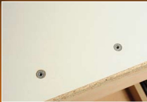
Metal fittings in the platen require precise fitting to locate with the vacuum cups in the frame
