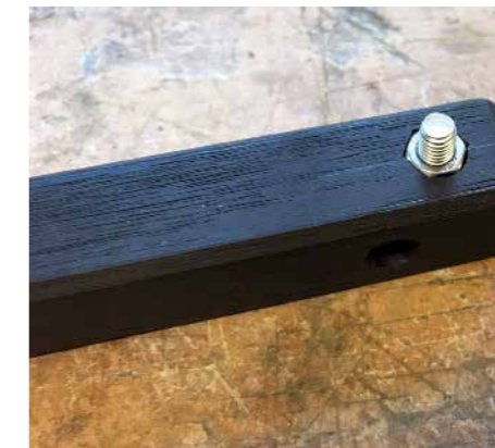
Sink the nut and the head of the bolt into the beam so they are flush
