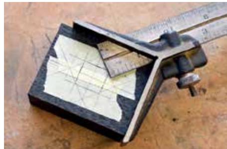
A 45° combination square is a great tool for generating accurate chamfers
