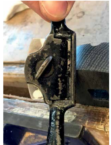
Soften all the edges with a chamfer
