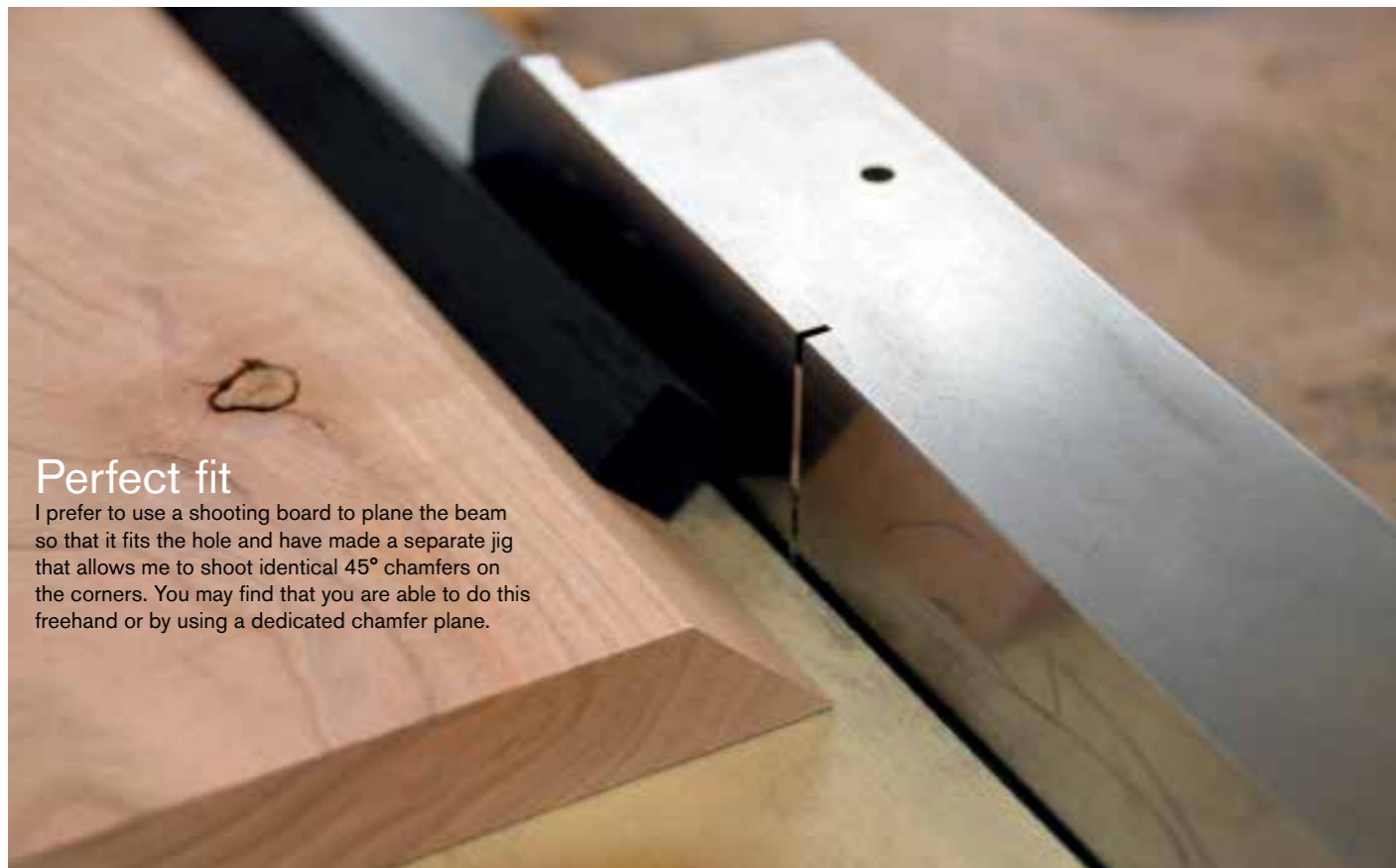
Convert your shooter to plane 45° with a simple jig
