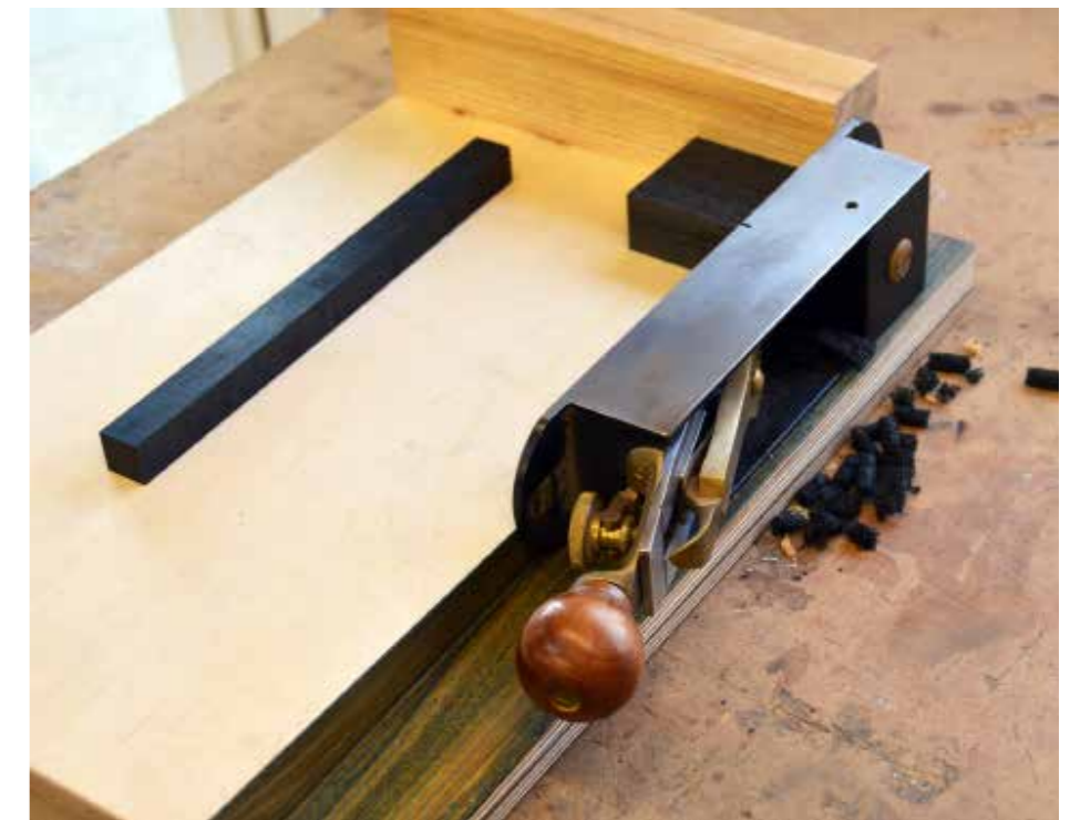
A shooting board is your best friend when it comes to dimension components by hand
