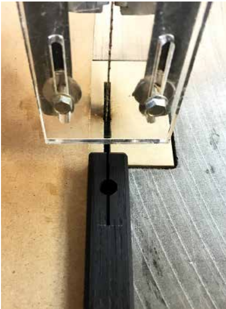
Cut a slot to give the clamp some spring
