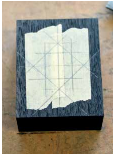
Use masking tape to highlight layout lines on dark timbers
