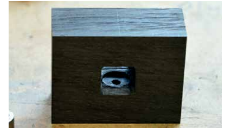
Create a recess to accommodate the washer
